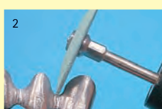
2 Non-precious and precious metal alloys The dtg grinders are perfectly suitable for processing of metal surfaces of ceramic frameworks thanks to the diamond coating.
