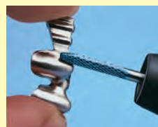
Fine cutting performance and smooth surface of the object: D292 KM 23 - application example in the precious metal technique
