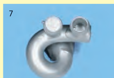
The considerable expansion of the competitor's resin during the incineration phase resulted in the fracture of the investment material die in the casting ring. After casting, the crown is sealed with a lid and can not be used. A section through the cast crown (figure 8) shows the fractured die.
