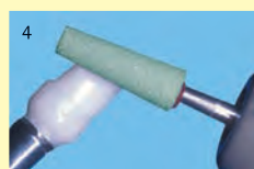
4 Rapid and convenient shaping of implant suprastructures. The fine diamond particles produce a smooth surface.
