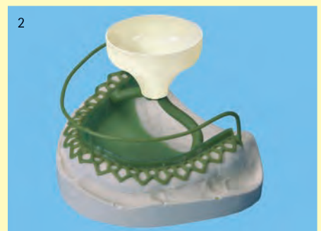
2 During casting the compressed air is displaced into the air channels and produces castings free from shrinkage cavities, which can be easily fitted.
