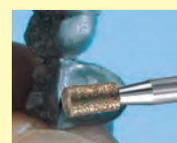
Finishing of deeper surfaces of metal frame-works.
