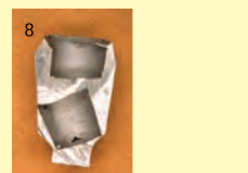
The considerable expansion of the competitor's resin during the incineration phase resulted in the fracture of the investment material die in the casting ring. After casting, the crown is sealed with a lid and can not be used. A section through the cast crown (figure 8) shows the fractured die.
