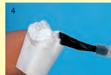
Gloss and hardening agent for plaster diffuses into the plaster so that it can also be used on the preparation margin.
