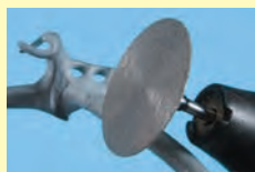
Separating and grinding back the sprues.
