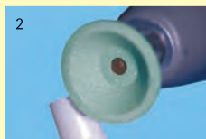
2 The inverted cone with recess provides a cooling effect and thus the perfect precondition for processing zirconium oxide.
